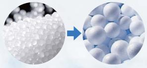
Raw material beads prior to foaming
